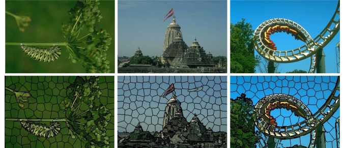
Fig. 1. Illustration of superpixel segmentation. Given an input image (top), the proposed algorithm groups the pixels into a specific number of small atomic regions (bottom).
